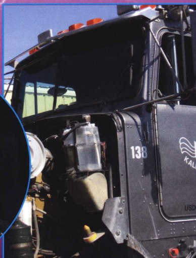
Hydrogen Generator Installed In a Dump Truck
